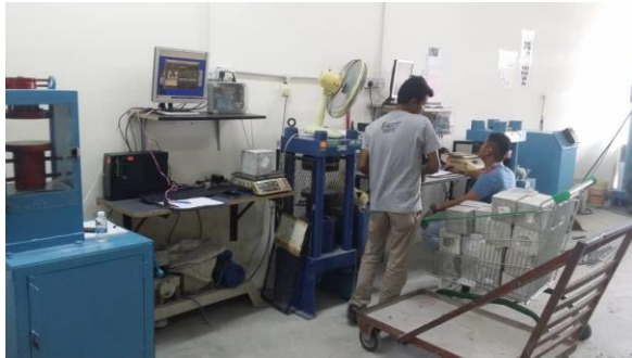
CONCRETE CUBE, BRICK AND CORE SPECIMEN DIGITAL COMPUTERIZED COMPRESSIVE STRENGTH TEST
