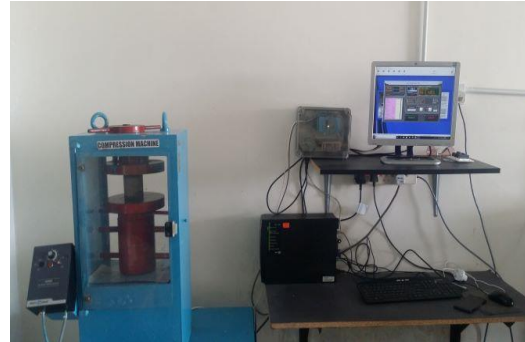
CONCRETE CUBE, BRICK AND CORE SPECIMEN DIGITAL COMPUTERIZED COMPRESSIVE STRENGTH TEST
