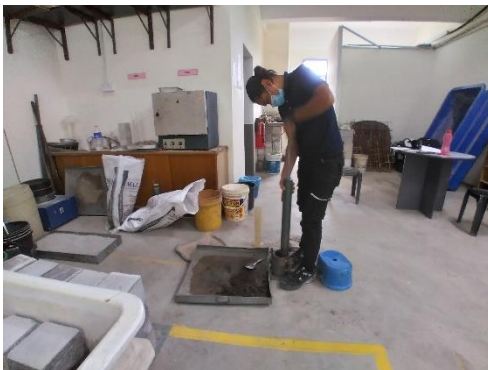
SOIL COMPACTION TEST
